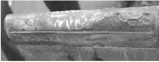
Fig. 14. View of rail CPS Li limiter after 'cold' plasma exposure.
